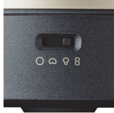
Figure 1: Selector for polar patterns
